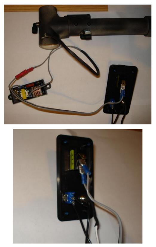
The next photos and drawing show the trigger/safety circuit.
