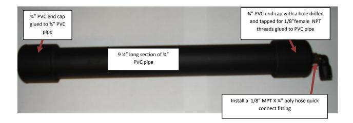
This concludes the work on the Gas Meter Tank assembly for now; we will resume work with it during the cannon assembly stage. Now is a good time to paint your cannon with the color scheme of your choice, if you so wish. (Be sure not to paint the Legris fitting.)
