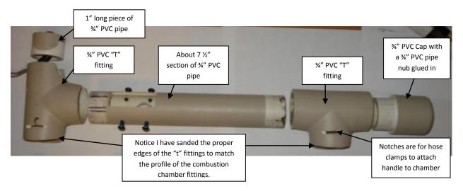
Note: Only glue the PVC pipe nub in to the cap. The disassembled joints in the photo above will remain unglued to allow for assembly and disassembly.
