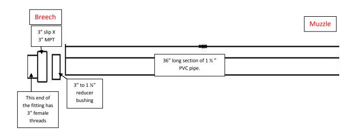
Here is a simple drawing of the barrel assembly to show the location of the fittings to allow for breech loading.
