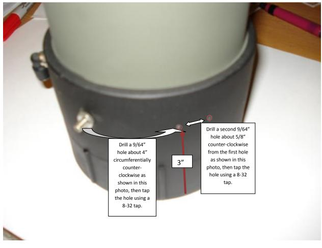
photo below. Drill the two holes as shown in the photo below, about 5/8" apart using a 9/64" drill and then tap the holes using an 8-32 tap.
