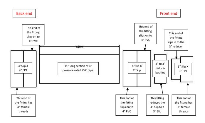
On the back end of the combustion chamber, you will need to glue a 4" Slip X 4" FPT (Female Pipe Thread) fitting. See photos below each instruction for details.
