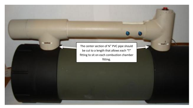
Now that you have the correct length of PVC cut for your handle, you need to create the cutout for the valve, and the bottom Legris swivel fitting, and then drill and tap the holes for mounting the valve. To begin, slide the PVC pipe into the front "T" fitting all the way and mark the depth on the PVC pipe. This
