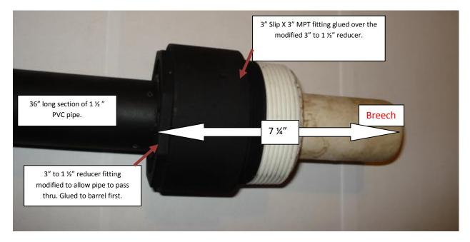
This concludes the work on the barrel assembly for now; we will resume work with it during the cannon assembly stage. Now is a good time to paint your cannon with the color scheme of your choice, if you so wish. (Be sure not to paint the large PVC fitting threads, as this will make them difficult to operate.)
