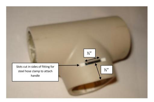
Fabricating the "T" PVC fitting for the front of the handle is next, and is similar to the back fitting you just fabricated. The difference is the orientation, notice in the photo below which edges need to be
