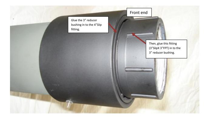
Your basic combustion chamber section is now complete and should look remotely like the one shown in the above pictures (minus the paint, plumbing, and electrical fittings which will be installed later).
