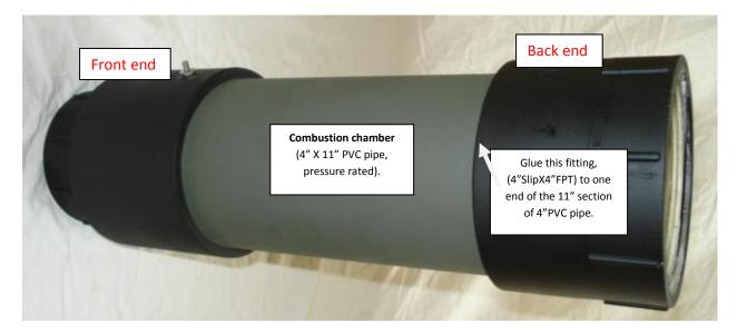
On the front end of the combustion chamber, you will need to glue a 4" Slip X 4" Slip fitting (this is a 4" pipe slip coupler, which would be used for coupling 2 sections of 4"pipe). Next, a 4" to 3" reducer bushing will be glued in to the 4"Slip fitting and reduce it to a 3" Slip fitting. Finally you will need to glue a 3"Slip X 3"FPT (Female Pipe Thread) to the reducer bushing installed in the previous step.
