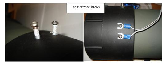
Now we will install the spark strip constructed earlier by clamping it between two nuts as shown in the photos below.
