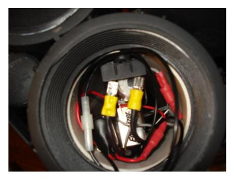
Now we will install the combustion chamber fan. First, install the ring terminals from the fan to the screws inside of the combustion chamber with 8-32 nuts and tighten. Then install the fan into the combustion chamber so that the air flows toward the muzzle end of the chamber.
