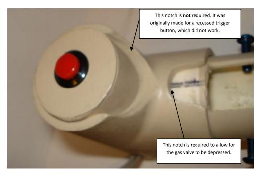
Go ahead and sub-assemble the handle to the level shown in the photo below in order to measure for the pipes that will be needed for the gas system construction in the next section.
