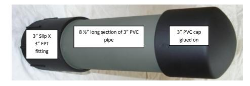
The first of the two pods just constructed will be used for a propane storage pod. The only thing you will have to do is modify a 3" PVC male threaded end cap by cutting out the center to allow for the propane bottle to protrude thru. I used a miter saw to cut out the square block in the PVC cap flush with the top of the cap. A drill and jig saw, hacksaw, or dremel would also work, use whatever you think you can make work best. The photo below shows the two caps required for the Storage Pods.
