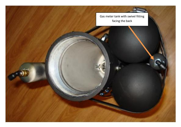
Once you get everything oriented to your satisfaction and all of the wires into the electronics pod, go ahead and tighten the hose clamps. You should now have one solid unit that can easily be carried using the handle.
