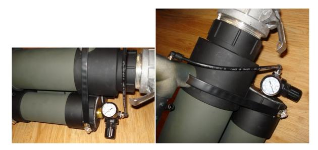
Cut another piece of ¼" OD poly tube the proper length to connect the swivel fitting in the bottom of your valve in the center of the handle to the swivel fitting in the combustion chamber and install the tube. Finally, cut another piece of ¼" OD poly tube the proper length to connect the swivel fitting in the back of the handle to the swivel fitting in the gas meter tank and install the tube. The photos below show the connection of the gas lines.
