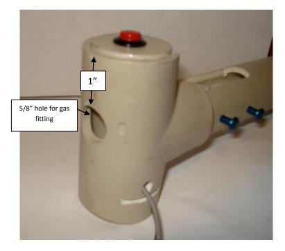
Next is the fabrication of the center section of the handle, it will be constructed of an approximately 7 and ½" long piece of ¾" PVC pipe. It should be verified that this is the correct length by dry fitting the pieces made above for the handle and ensuring it fits on the combustion chamber as shown in the photo below.
